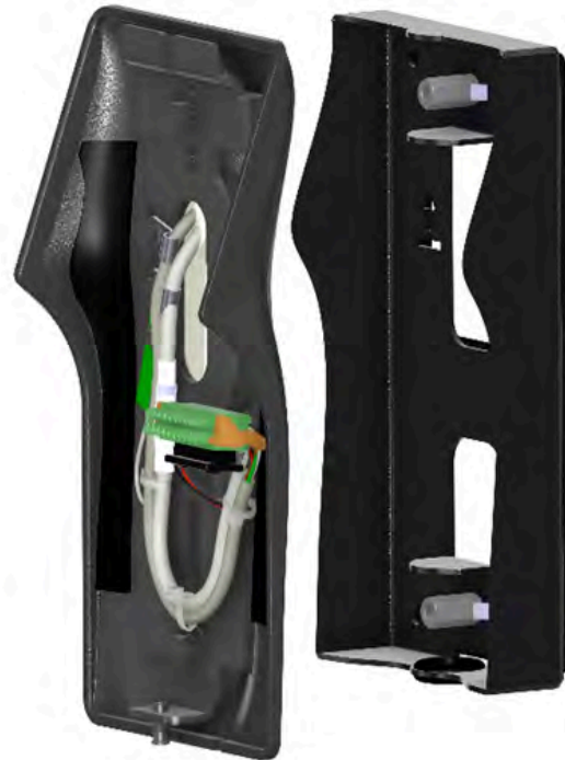
Flowbird Axio on-board validator, with a wall mount adaptor.
