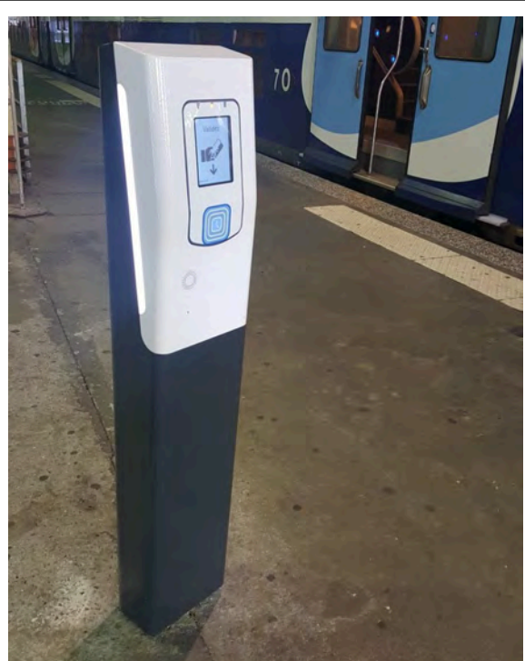
Axio PV platform validator at SNCF (French railways)
