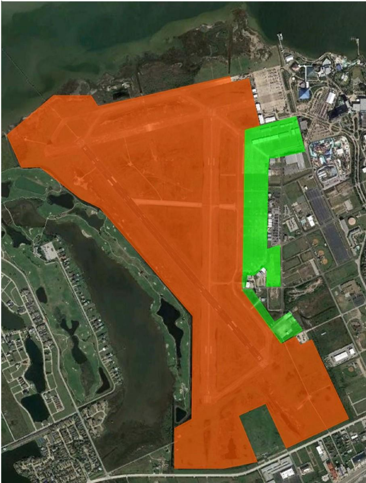
SCHOLES INTERNATIONAL AIRPORT Figure 1 – Airport Operations Area (AOA) AOA INCLUDES MOVEMENT AND NON-MOVEMENT AREAS
